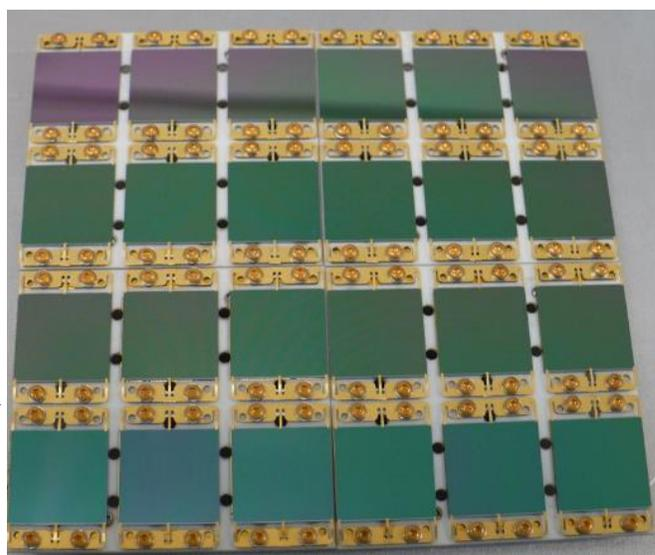
SiPM covered barrel (4 m<sup>2</sup>) for scintillation light detection
